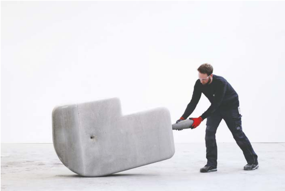
Fig. 10. Removing counterweight to stand element.
